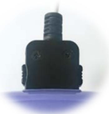
Plug the connector into the transmitter with the arrows facing the back clip and **the screws facing the front**. Be sure to push the connector in until it clicks.
